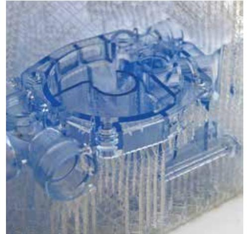
*"e-Stage enables us to orientate components in ways that traditionally would have been unimaginable. We can now nest/overlap parts in Z as e-Stage grows supports around surfaces to minimize the number of contact points. This combination allows our company to optimize build quality and maximize build capacity. Overall, the improved build quality dramatically reduces part finishing ultimately saving money, but more importantly helping to maintain our reputation for part quality."*
